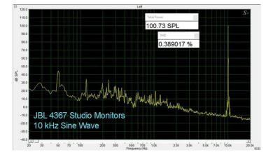
Distortion measurements for speakers are typically done at a 90 dB reference point but the distortion numbers for the JBL 4367s were low enough that I also measured them at 100 dB to really see what these drivers could do. This is considered loud by any stretch and some lesser drivers would balk at these levels. This particular graph shows a distortion level at 10 kHz of only 0.389017% at 100 db. Essentially inaudible.
