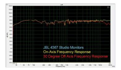
This chart shows the on-axis frequency response directly compared to the 30 degree off-axis measurement. The two plots track each other tightly until we get to about 13 kHz where the treble energy begins to gently roll off.
