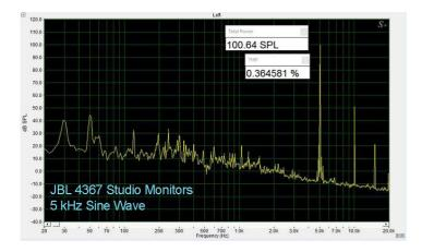
At 5 kHz the distortion level at 100 dB is lower still, at 0.364581%. Also, inaudible.
